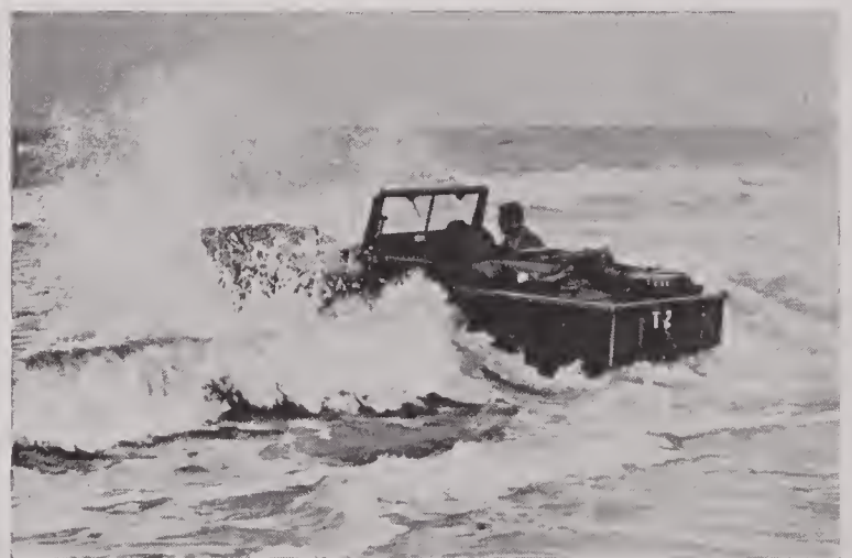
FIGURE 5. In moderate surf, early pilot model of Ford amphibious jeep impressed military observers. Production models were not waterproofed, and the engines drowned out.
